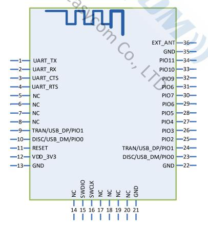
Figure 3: FSC-BT986 PIN Diagram(Top View)
