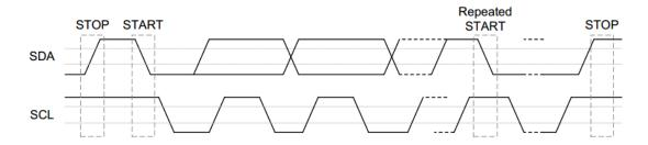
Figure 5: I2C Bus Timing
