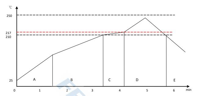
Figure 6: Typical Lead-free Re-flow
