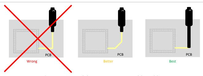
Figure 12: Recommended Trace Connects Antenna and the Module
