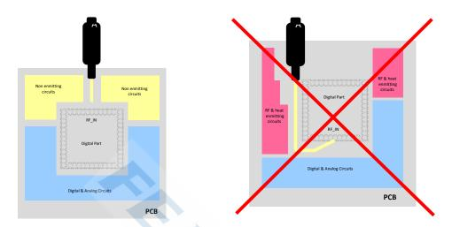
Figure 10: Placement the Module on a System Board
