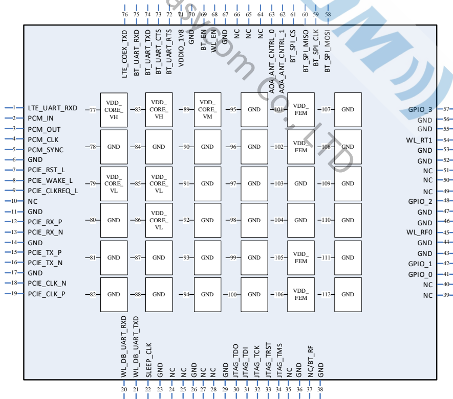
Figure 3-1-2: FSC-BW1001UV PIN Diagram (Top View)
